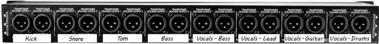
**ART S8 3-way mic splitter** is the top-most piece in the band's IEM rack. All microphones on stage will feed directly to a 9 input snake (provided by the band) which feeds the ART splitter in the IEM rack. An additional 8-channel snake will feed directly from ART splitter to house snake for FOH mixing. The splitter provides a clean mic signal for all FOH inputs. **The band will take care of the IEM mix.**
